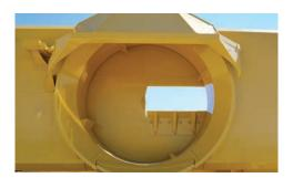
JOBSITE SAFETY. The thrown object restraint system (TORS) reduces the amount and distance of thrown material debris and has a smooth underside for optimal material flow.
