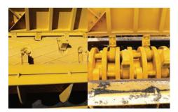
**OPTIMAL CUTTING PERFORMANCE.** The patented Series III duplex drum offers proven cutting performance and reversible hammers and tips nearly double the wear life of single-sided designs, simplifying daily maintenance.
