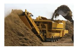
PRECISE PLACEMENT. A radial stacking rear discharge conveyor oscillates 60 degrees, allowing the operator to place the processed material where they need it without moving the machine.
