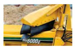
THROWN OBJECT DEFLECTOR (TOD). Reduce the quantity and distance of thrown material debris with the TOD, strategically placed to reduce interference when loading over-length material.
